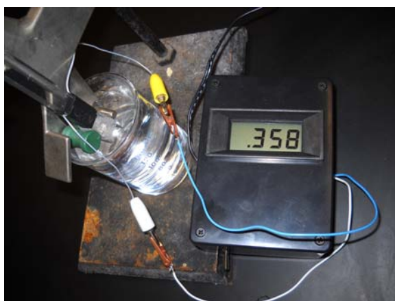
Figure 1. Student constructed conductivity meter.
